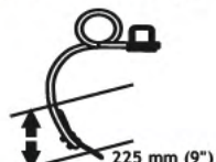
225 mm (9") Dent double ressort en acier type EN-45
