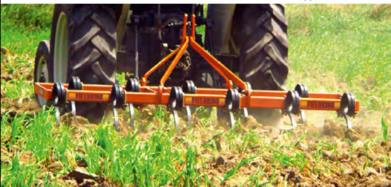
225 mm (9") Dent double ressort en acier type EN-45
